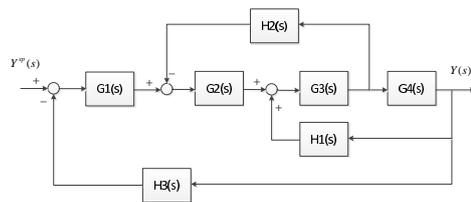
$$G_1(s) = \frac{1}{s+10} \quad G_2(s) = \frac{1}{s+1} \quad G_3(s) = \frac{s^2+1}{s^2+4s+4} \quad G_4(s) = \frac{s+1}{s+6}$$
